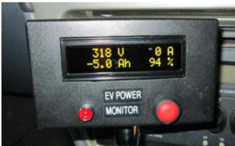
The BCU has two display modes, just press and hold the monitor button to toggle between them. This button may also be pressed to reset any error conditions.
