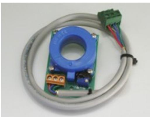
The current sensor is a non contact Hall effect type. It can accurately measure up to +/- 300A. Larger currents are allowed but will be measured at the maximum level only.
