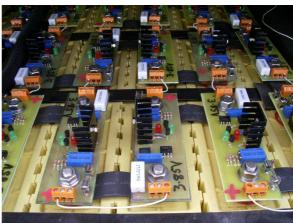
The first time I installed the BMS it worked! And it continues to work after dozens recharges. I halved the weight of my battery pack, increased the performance and doubled the effective range of my little EV to 60-90km. The battery lifetime? Well that is to be determined. It now has done several thousand km on the LiIon pack with no signs of ageing. I would hope for at least 50000km useful life. Of course the system costs about five times as much as Lead Acid but I for one will never go back.
